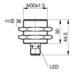
**Inductive Sensors** BES 516-3028-E5-Y-S 4 M30x1.5 x 44.5 normally-closed Sn=10mm shielded
